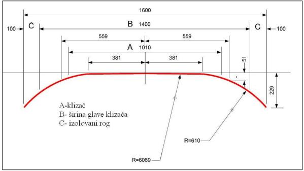
Figure No 1. – Dimensions of pantograph
